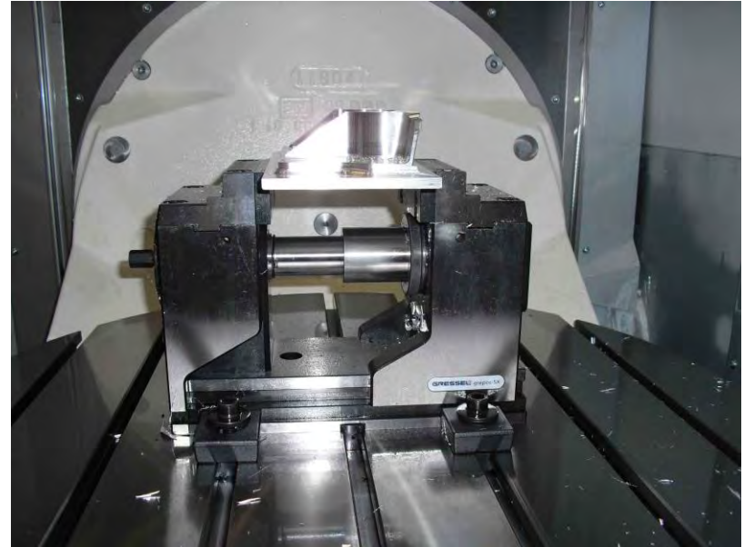
Gressel Grepos 5 X, BB125 mm, height 214 mm
